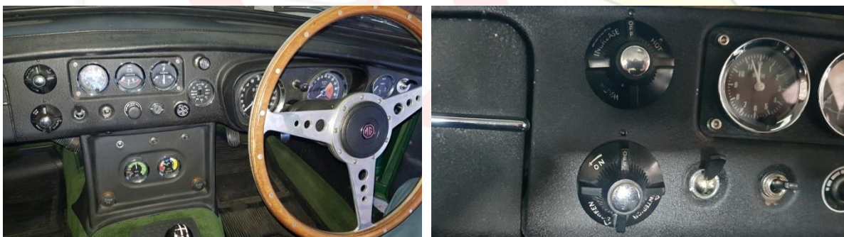
ABOVE LEFT: MG dashboard and console RIGHT: Heater controls, temp-top, direction-bottom
